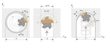
TSC milling (right) is a combination of circular milling (left) and full-slot milling (center).
